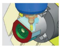
You can see the G-code rotary angles update while the simulation runs in the NC Program window within the Simulation Control Panel dialog box.
