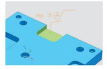
This plate also has surface finish PMI attached to the floors and walls of this pocket. NX CAM can recognize it and use it to automatically determine the selection and definition of machining operations.
