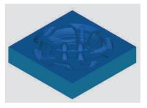
The material removal option provides visualization of the actual results you would expect when machining the part.
