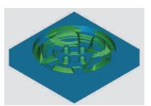
While the verification plays, note that the smaller tool used for the rest mill operation only machines the areas where the previous roughing operation left uncut material.
