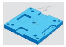
The plate appears in the graphics window. It is a solid body and does not contain any parametric features. NX CAM can recognize and create machining features directly from solid bodies.
