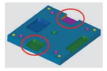
As the tool paths verify, notice that the pocket with the surface finish PMI is machined using additional operations compared to the mirrored pocket on the other side of the part.
