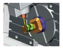
Fast and accurate roughing and finishing methods facilitate machining of complex parts, such as those typically machined for the aerospace industry. Z-level method with tilted tool facilitates the use of shorter tools to reduce tool deflection. Smooth flowing Streamline strategy is an ideal cutting method for multi-axis HSM finishing.
