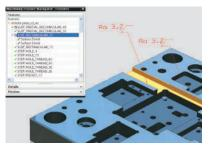
Each machining step is selected using configurable logic and criteria managed in a machining database provided as a part of the system. You can easily configure, add or modify the feature-based machining operations and how they are selected using a simple editor (Machining Knowledge Editor).
