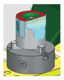
The tool path is displayed. See how it follows the natural shape of the freeform area of this part. This smooth flowing tool path is an ideal cutting strategy for multiaxis machining because it can produce a superior surface finish at a high feed rate.
