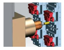
Fully automated rest milling removes uncut material from previous operations and eliminates
