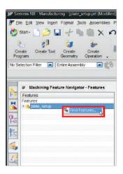
In the Machining Feature Navigator, right-click on the plate\_setup feature group, then choose Find Features.
