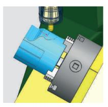
As the operations are simulated, the in-process workpiece (IPW) is passed from one operation to the next so that each subsequent operation can begin machining based on the IPW of the previous operation. This allows you to see an accurate representation of the workpiece's shape as the NC program progresses.
