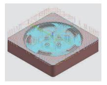
The new roughing operation with the trochoidal cut pattern is displayed.
