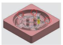
As the tool path verifies, note the sharp corners as the various cut levels are displayed. These sharp corners can overload the tool and may cause early tool failure.
