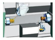
Keeping track of the in-process state of the workpiece is a critical component of effective millturning. NX CAM automatically generates an in-process workpiece (IPW) to provide seamless transfer of workpiece configurations between milling and turning.
