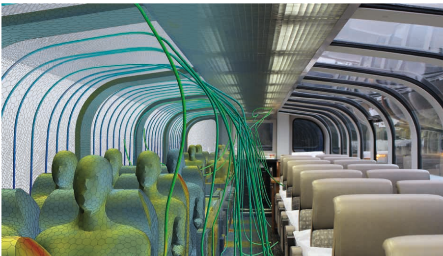
Digital twin of a train cabin developed by Stadler Altenrhein AG in STAR-CCM+ to improve passenger thermal comfort.
